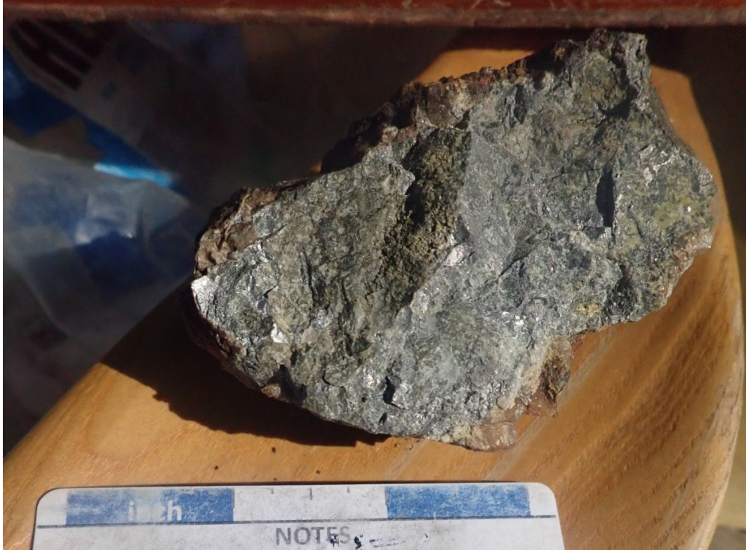
Figure 7: massive arsenopyrite float, weathered out of the Damocles Vein (Hodgson Island). This sample returned 2.28 g/t Au; however, most of the structure was barren bull quartz-carbonate
