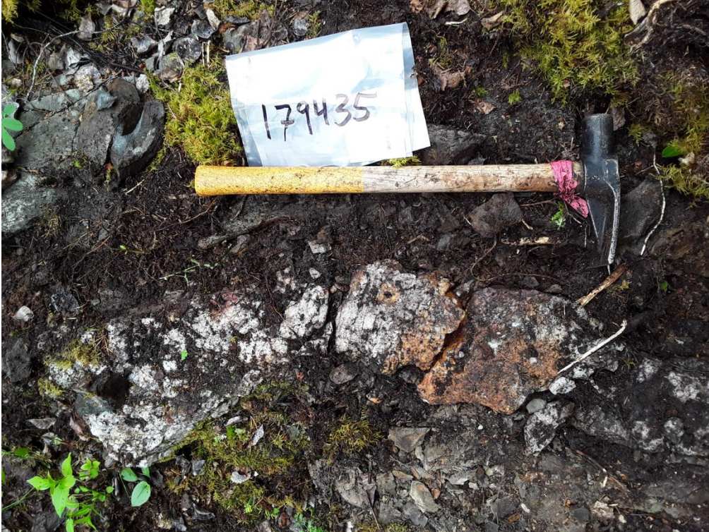
Figure 18. Sample 179435 returned the highest gold result from the 2020 exploration program of 2530 ppb Au. This sample was collected from a 25 – 30 cm quartz vein striking AZ 160 / dipping 65.
