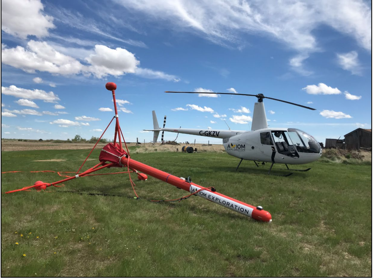
Figure 6: Helicopter & Triaxial Surveying Setup
