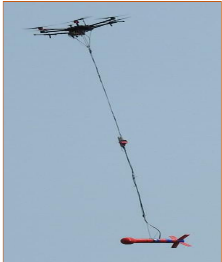
Figure 9. Devbriio UAV-Multirotor with CS-VL magnetometer.
