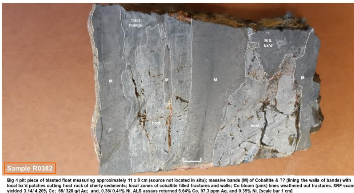
Figure 6. Cut Muck Sample of Cobaltite Vein Showing Internal Features. The in-situ source was not located by stripping.
