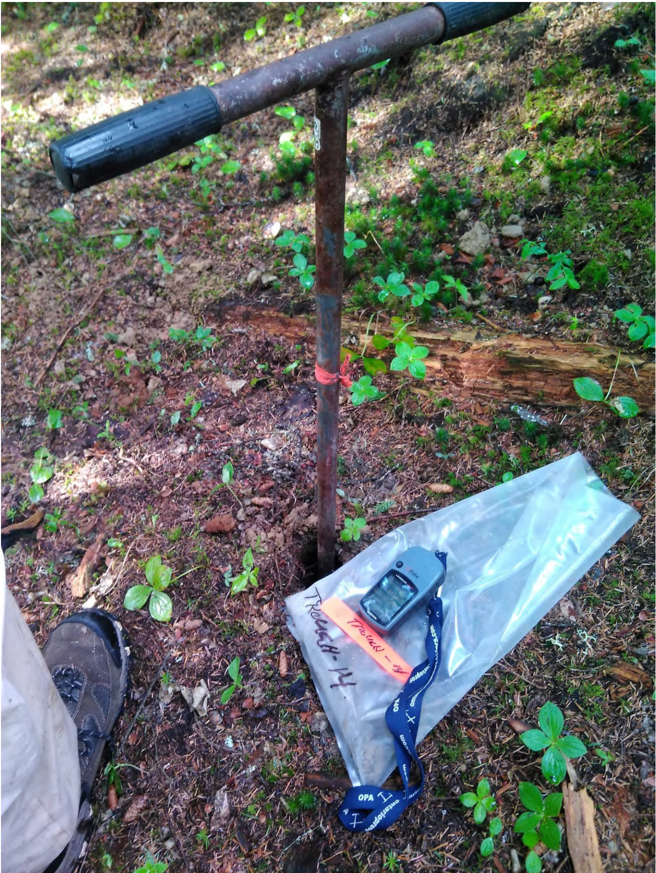
Sample Trough 14. Photo shows maximum depth sample could be taken without damaging the sampling tool.
