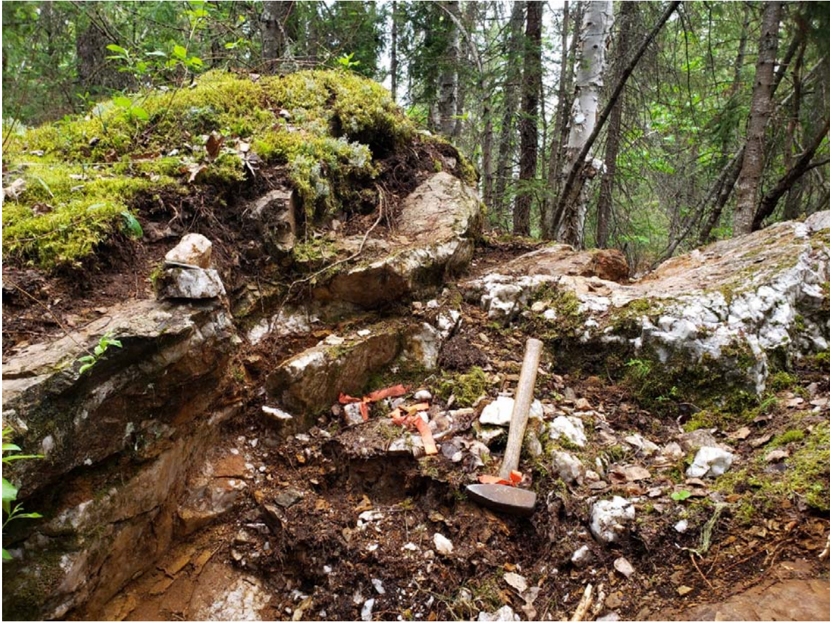
Photo 10: Pit 9 at LSG-5 sample site; 2-5cm white quartz-carbonate vein trending at 200/30 in strongly fe-carb-sericite-pyrite-altered mafic volcanic; looking northeast; Sample 1475910 taken from west wall; veins “roll” in pit and can be flat lying to gently dipping
