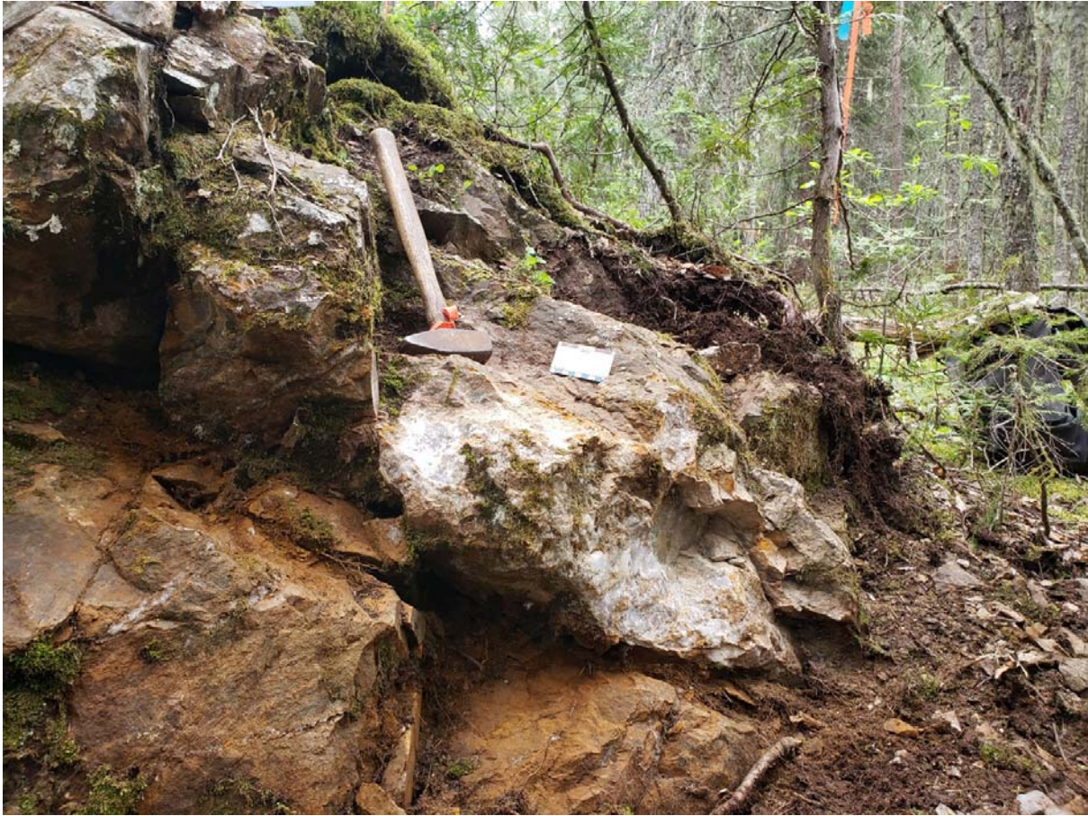
Photo 12: Old pit; 50cm white quartz-carbonate-chlorite vein stockwork in moderate fe-carb-chlorite-altered mafic volcanic; looking southeast; Sample 1475912
