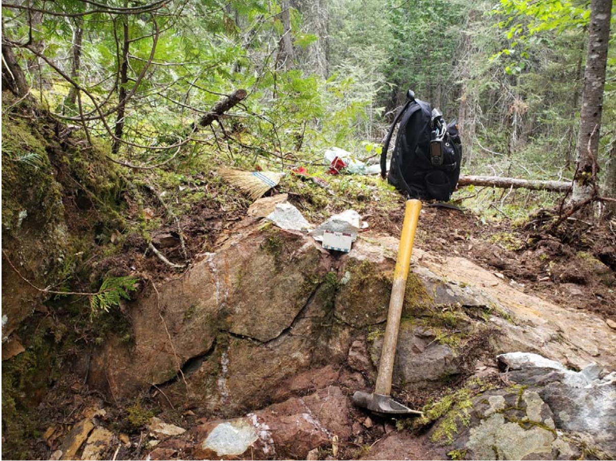
Photo 13: Old pit on outcrop at edge of swamp; 1-2cm white quartz-carbonate veins and stockwork trending at 320/90 in intensely fe-carb-sericite-altered mafic or felsic volcanic; looking north; Sample 1475913
