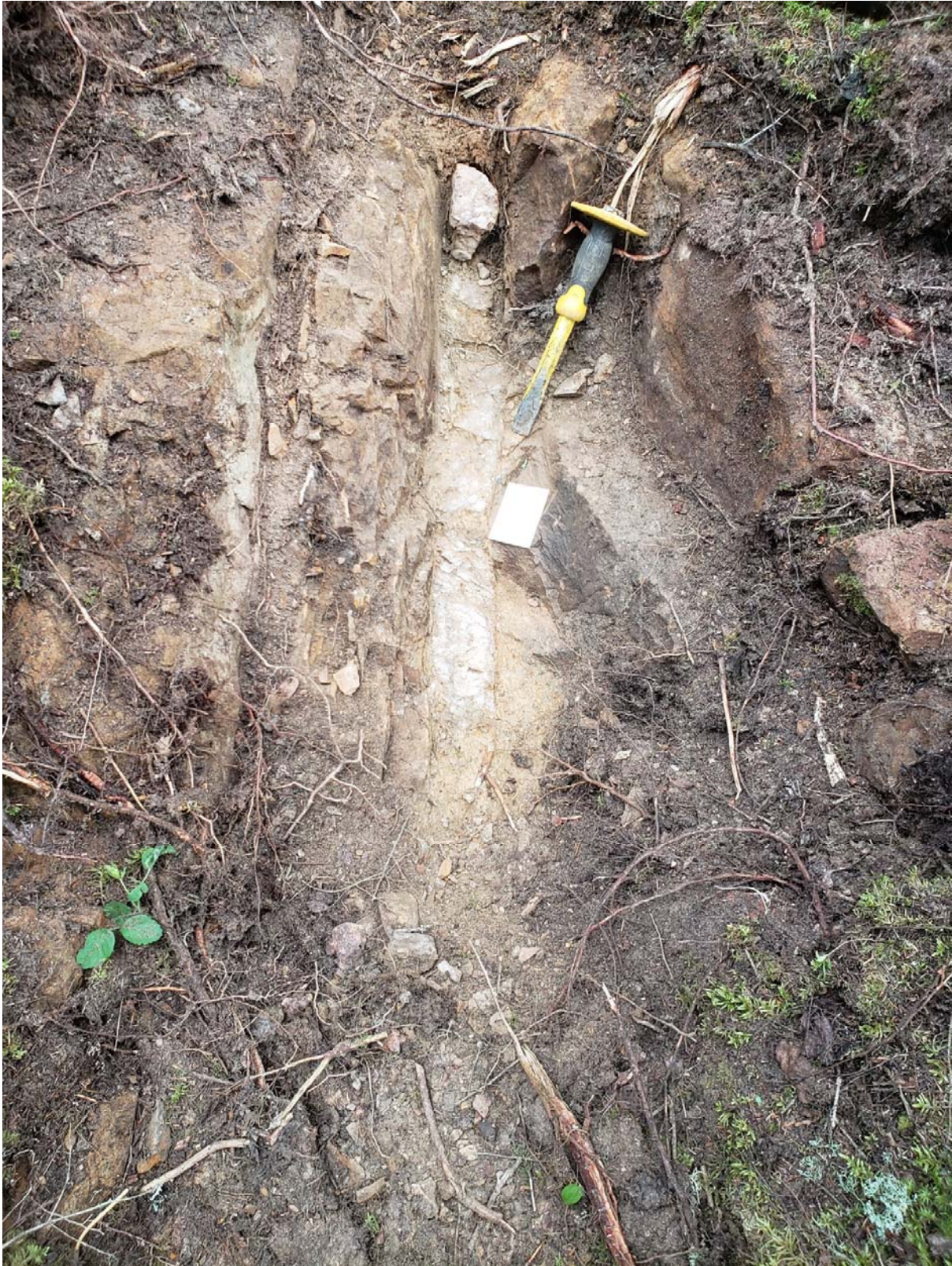
Photo 7: Old trench approximately 25m northwest of shaft 1; 10cm white quartz-carbonate vein trending at 320/80 in well foliated fe-carb-altered mafic volcanic; looking northwest; Sample 1475902
