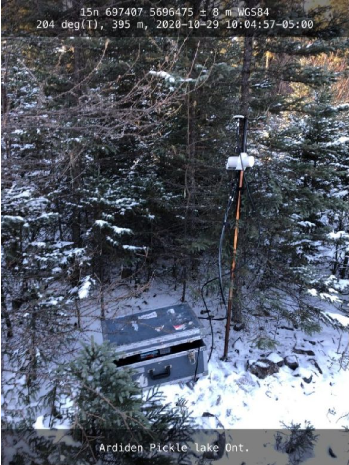
Figure 4: Base station setup
