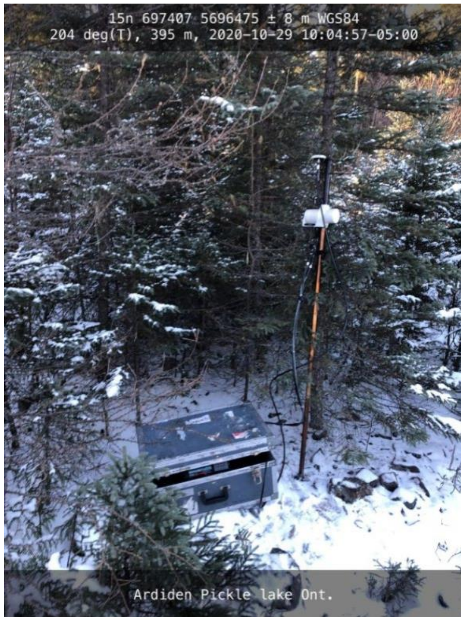
Figure 7 – Base Station Setup
