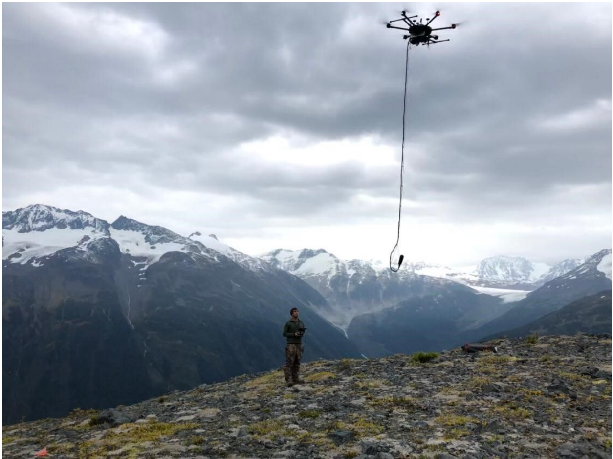
Figure 5: UAV Magnetometer System Configuration
