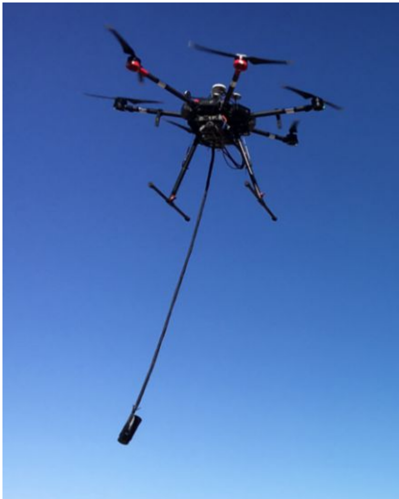
Figure 5: UAV Magnetometer System Configuration
