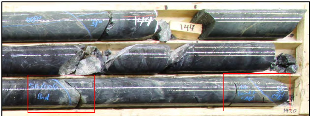
Plate 1. Core photograph from LXB20-001 at 146-147m depth. Note the beige-coloured alteration bands on the bottom section of core; likely represent pillow margin features.
