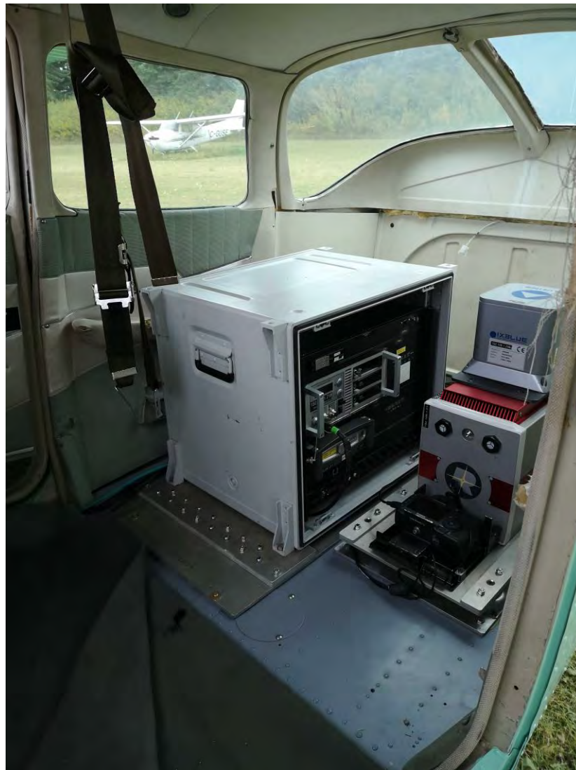
Figure 2: Q780 Laser, IMU and Computers Mounted in Cessna 182
