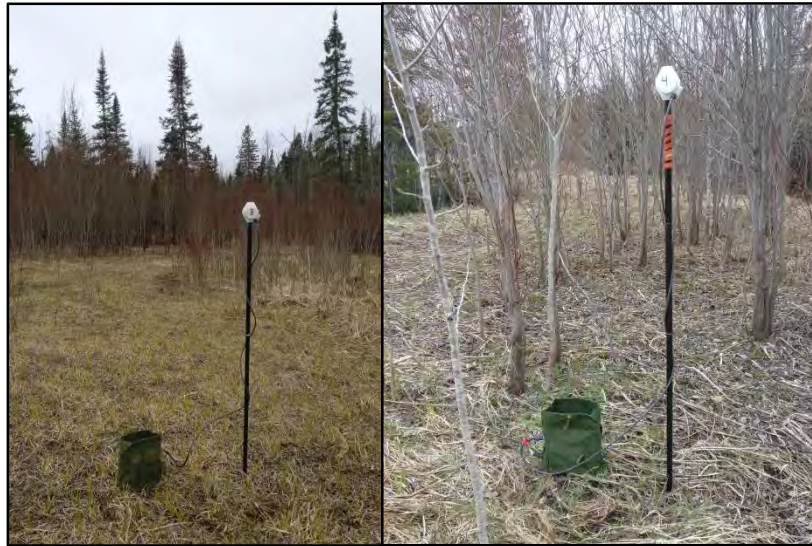
Figure 15: GEM 3 (left) and GEM 4 (right) magnetic base stations at Cochrane, Ontario.
