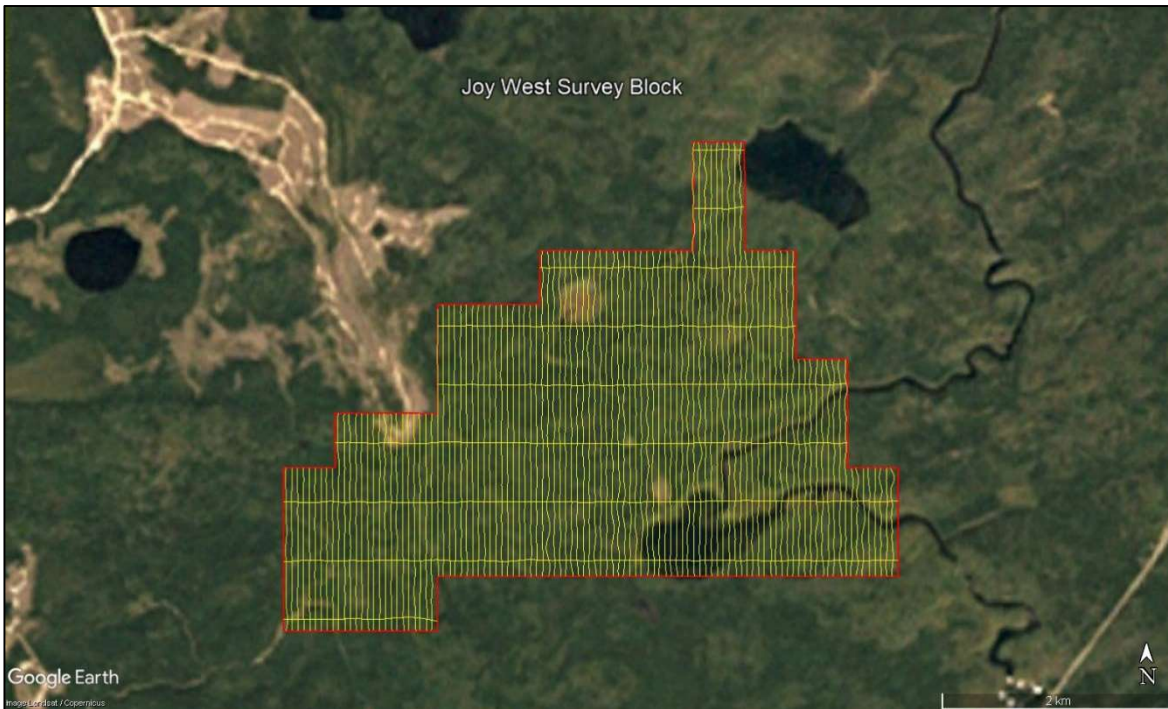
Figure 3: Plan View – Joy West survey block with actual flight lines in yellow and survey block boundary in red.
