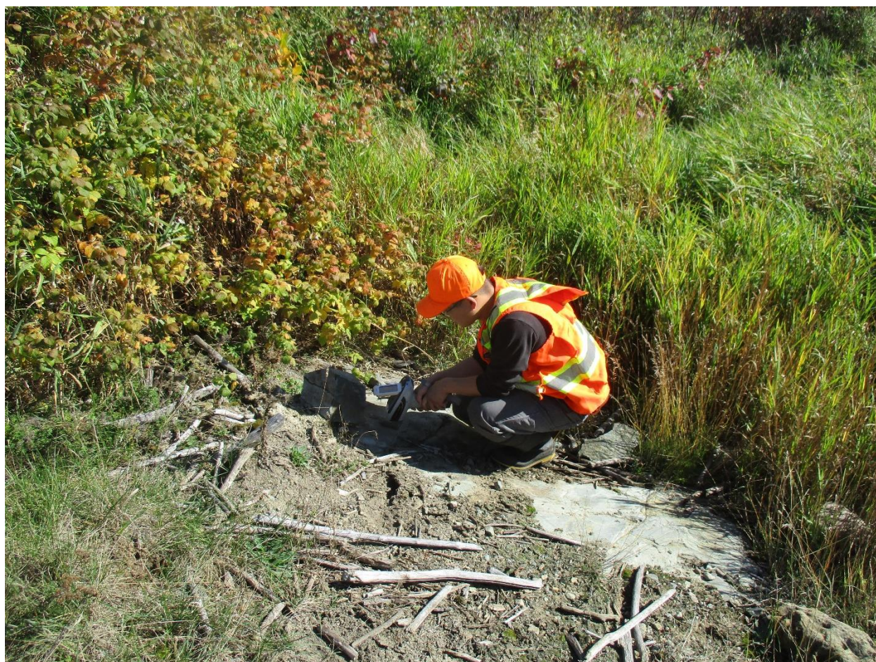
Figure 3: Field image of personnel conducting pXRF analysis
