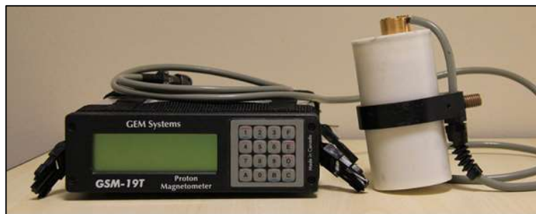
Figure 13: GEM GSM-19T proton precession magnetometer.
