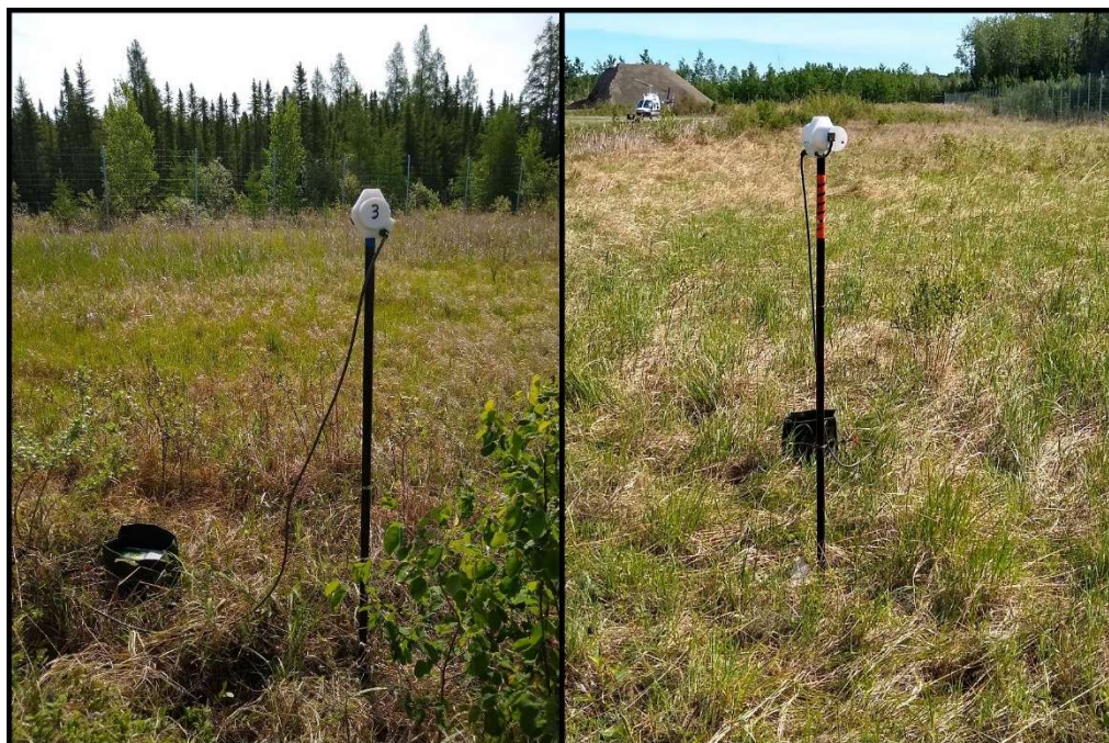
Figure 15: GEM 3 (left) and GEM 4 (right) magnetic base stations at the Red Lake Airport, Ontario.
