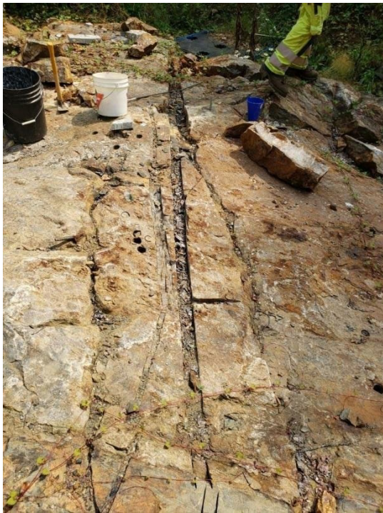
Figure 5. Exposed outcrop with disseminated sulphides. Channel sampling was performed on outcrop.
