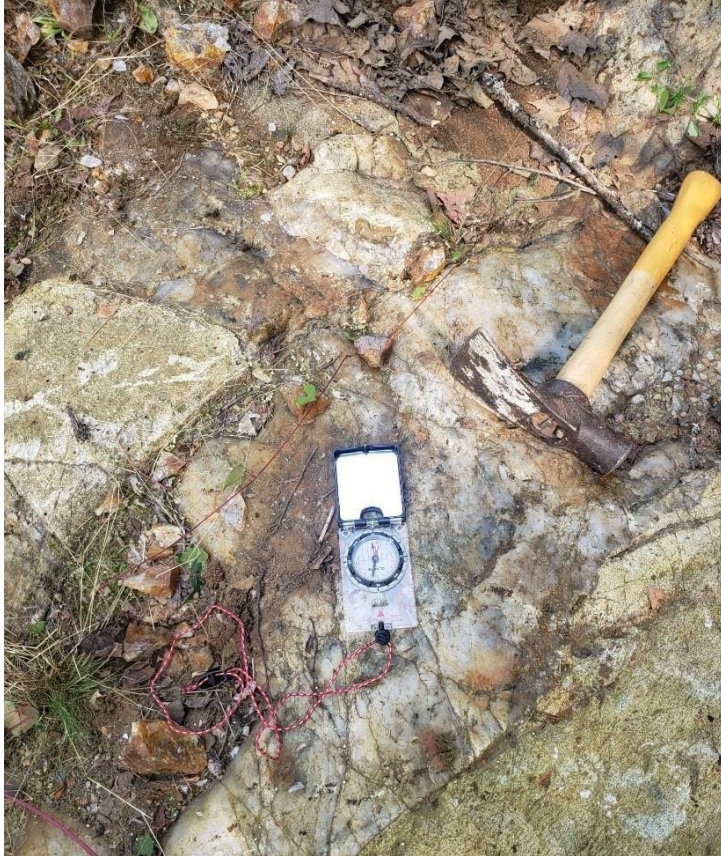
Figure 6. Quartz vein with sulphide staining and pyrite blebs exposed during excavation. Compass facing north.
