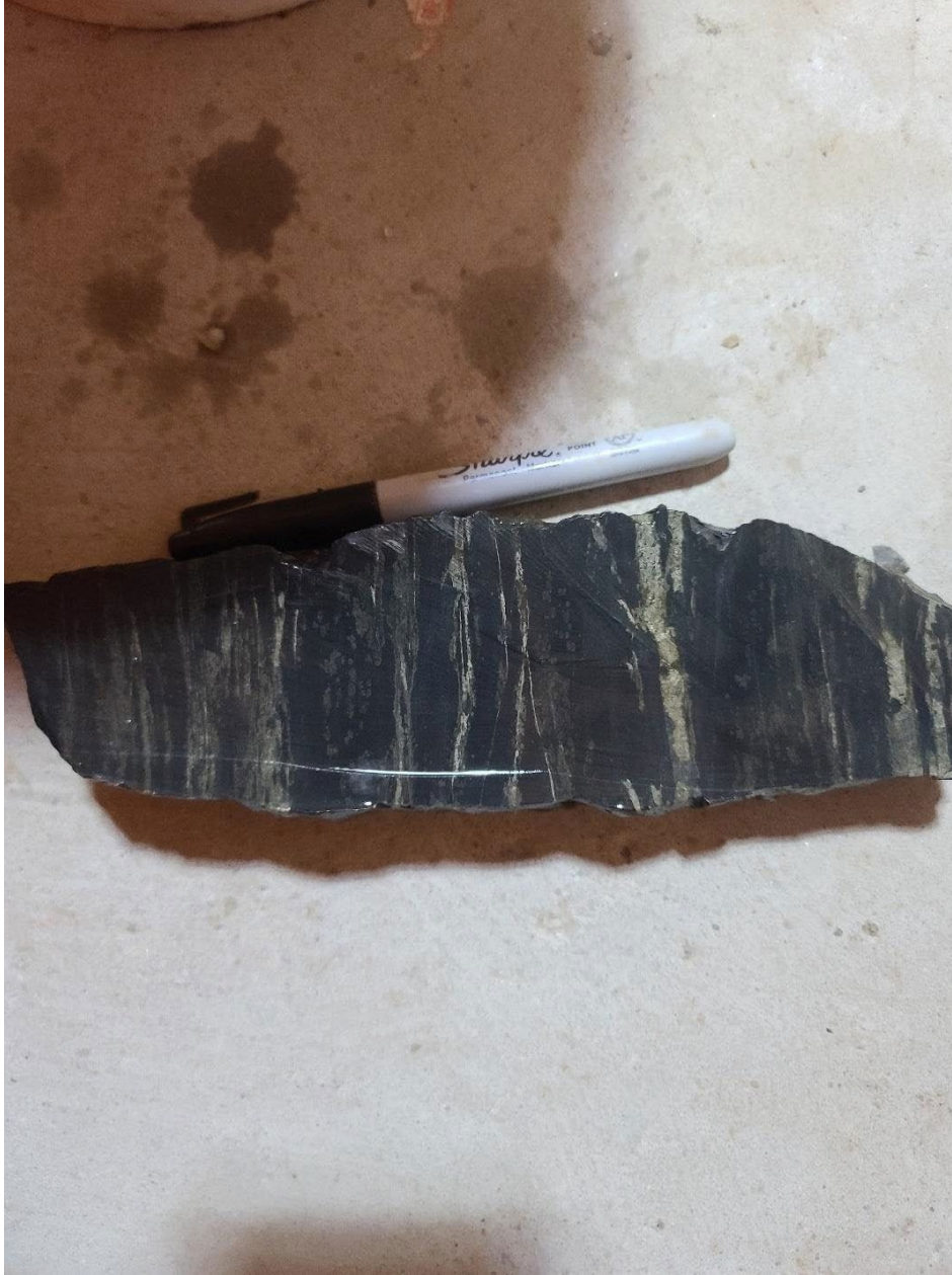
Figure 7. Black shale with pyrite in quartz veins obtained from lean iron formation
