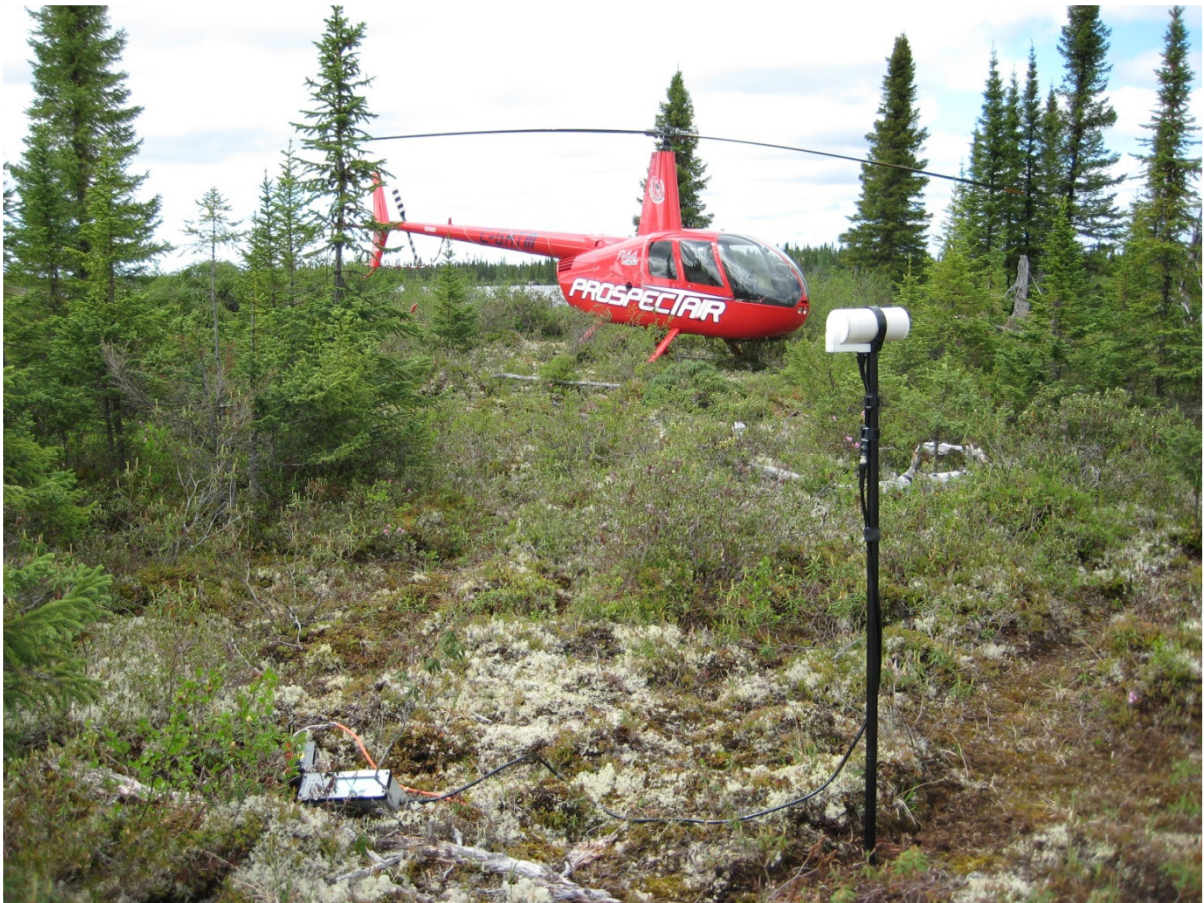
Figure 5: Example of a magnetic base station setup
