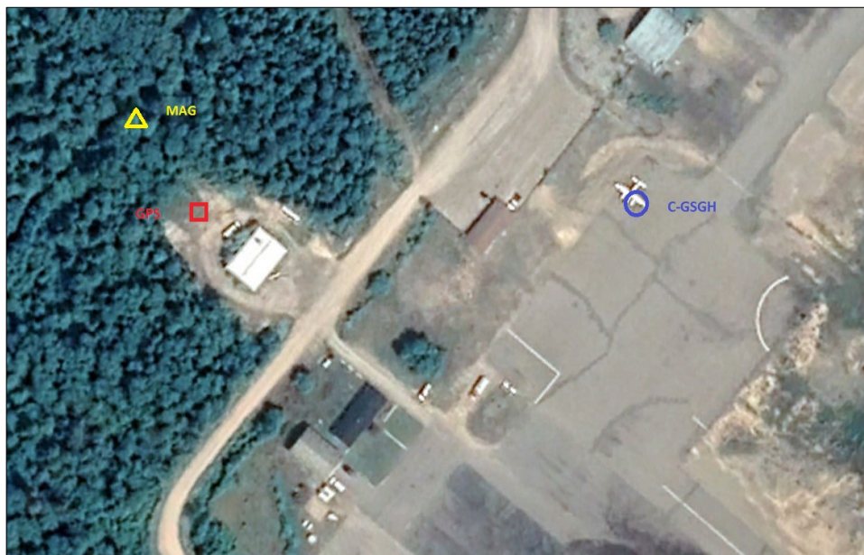
Figure 4: Location of the mag sensor (yellow) and GPS antenna (red) for the reference station, Gnd1 at Chapleau airport, and also the parking position of the helicopter C-GSGH (purple).
