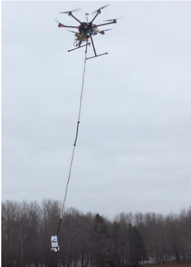
Figure 7: Magnetometer sensor suspended below platform with a 5 m tether
