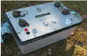
Extension Switch Pro box able to drive 24 - 48 - 72 or 96 electrodes
