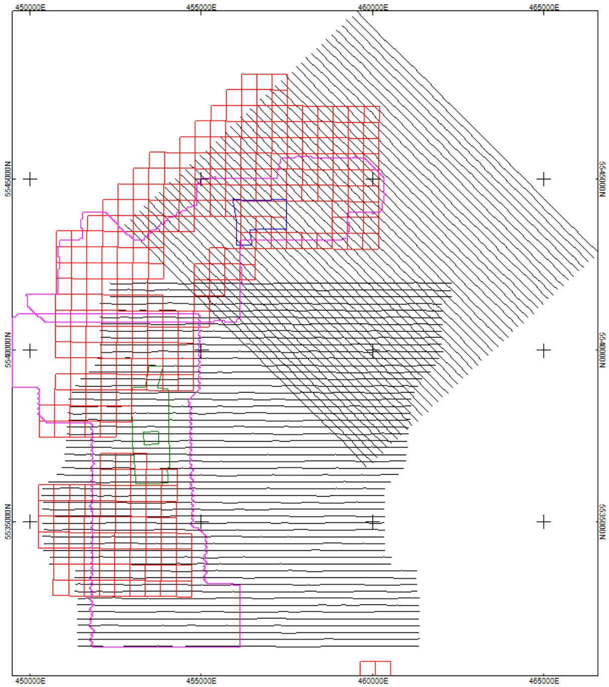
Figure 3 ZTEM flight lines (black) over tenure and outlines (magenta) of the HeliGOTEM II surveys
