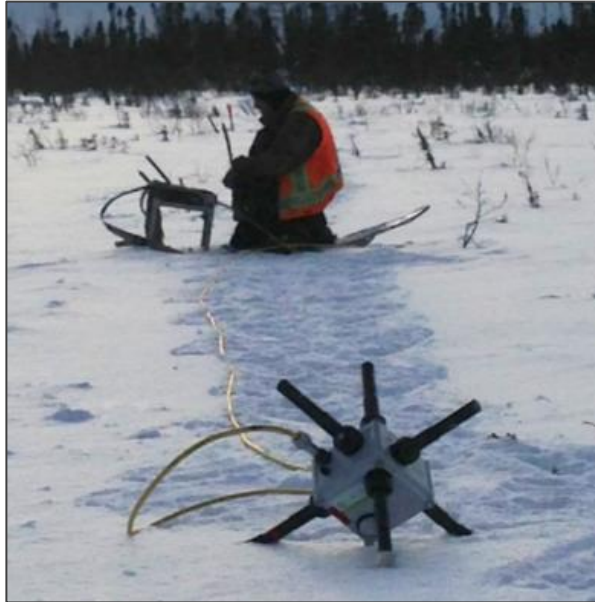
Figure 30. ARMIT Mk2.5 Probe in the Field.
