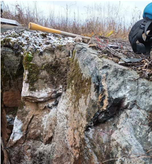
Figure 5: Photo of Aplite Vein in NW corner of shaft, Looking West. Chip Sample #2 taken across aplite vein mid-height of photo. North wall of shaft (right side of photo) has significant cobalt bloom in diabase.
