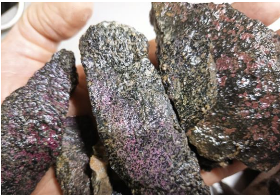
Figure 6: Diabase grab samples from north wall of shaft. Cobalt bloom through approximately 2 inches of diabase on footwall side of vein.
