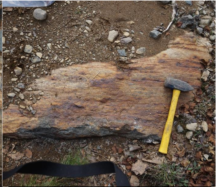
Sample 21DCHL004 Metasediment with semi-massive sulphides
