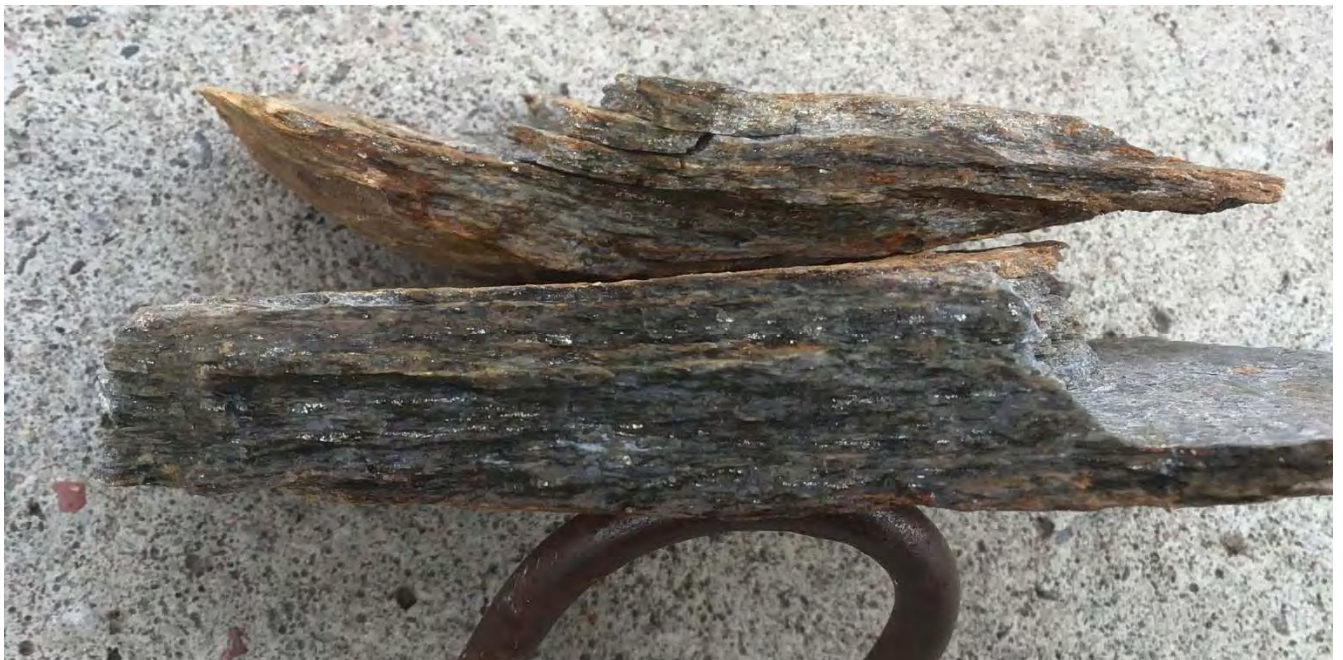
Photo 18: Silicified, sericitized and pyritized <30cm shear zone in intermediate volcanics. Fine grained pyrite and minor chalcopyrite in 1mm foliation parallel bands. Sample D295226. 634253/5580882.
