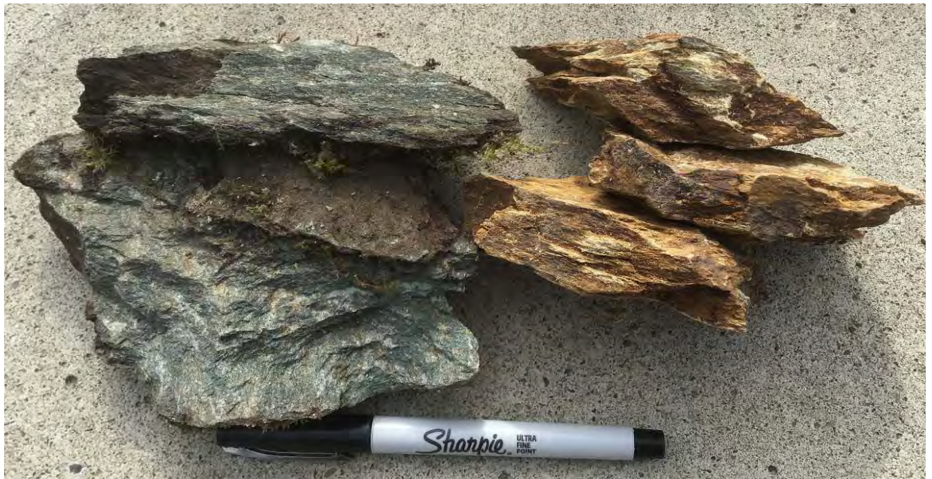
Photo 38: Rusty pyrite-magnetite bearing chlorite-sericite-carbonate altered psammities. D295234 & D295235.
