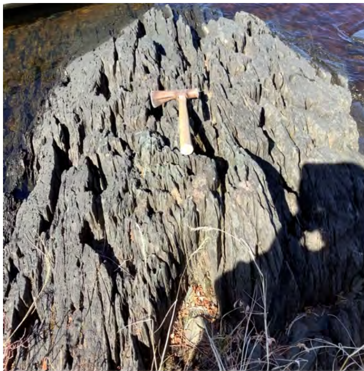
Photo 20: Strongly sheared chloritic mafic volcanics. 648244/5583190.
