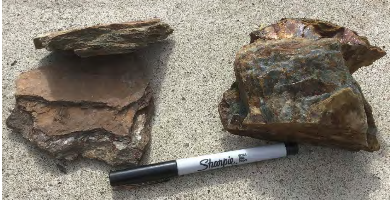
Photo 37: Rusty pyrite-magnetite bearing chlorite-sericite-carbonate altered psammities. D295233 & D295238.
