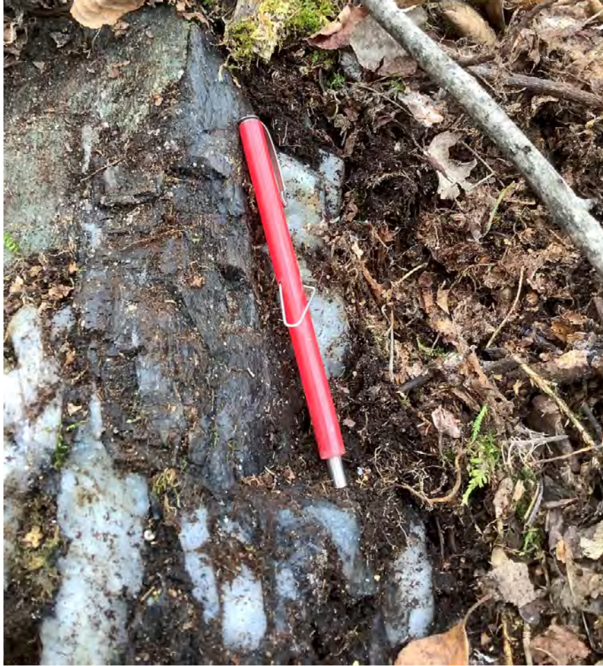
Photo 47: Barren quartz-coarse tourmaline vein in mafic volcanics. 634788/5580361.
