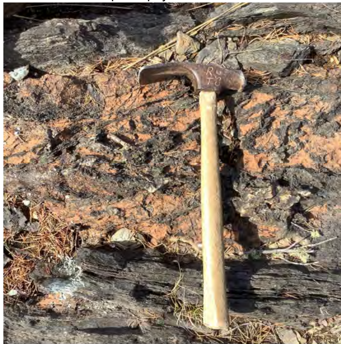
Photo 30: Sheared mafic volcanic with Fe-carbonate pod stockworked by quartz veining. 634636/5580745.
