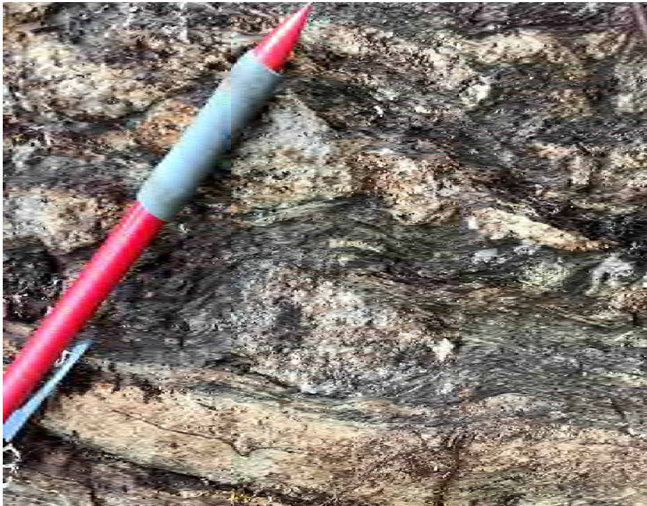
Photo 54: Dextral shear tails on tonalite clast in conglomerates. 632882/5581261.
