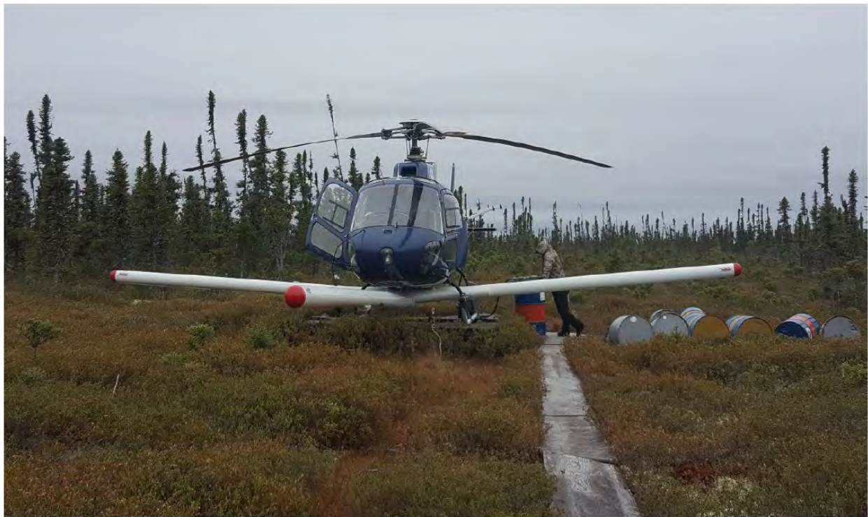
Figure 8-1 Photo of Terraquest’s tri-boom multi sensor helicopter with 3 magnetometers.
