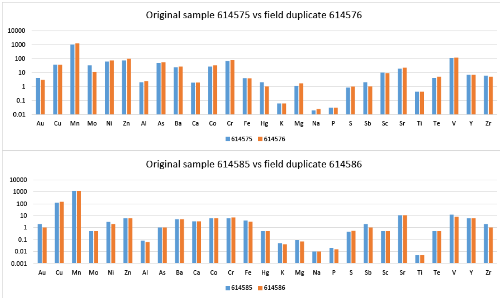
Fig. 15: Selected elements in original samples compared to field duplicates.
