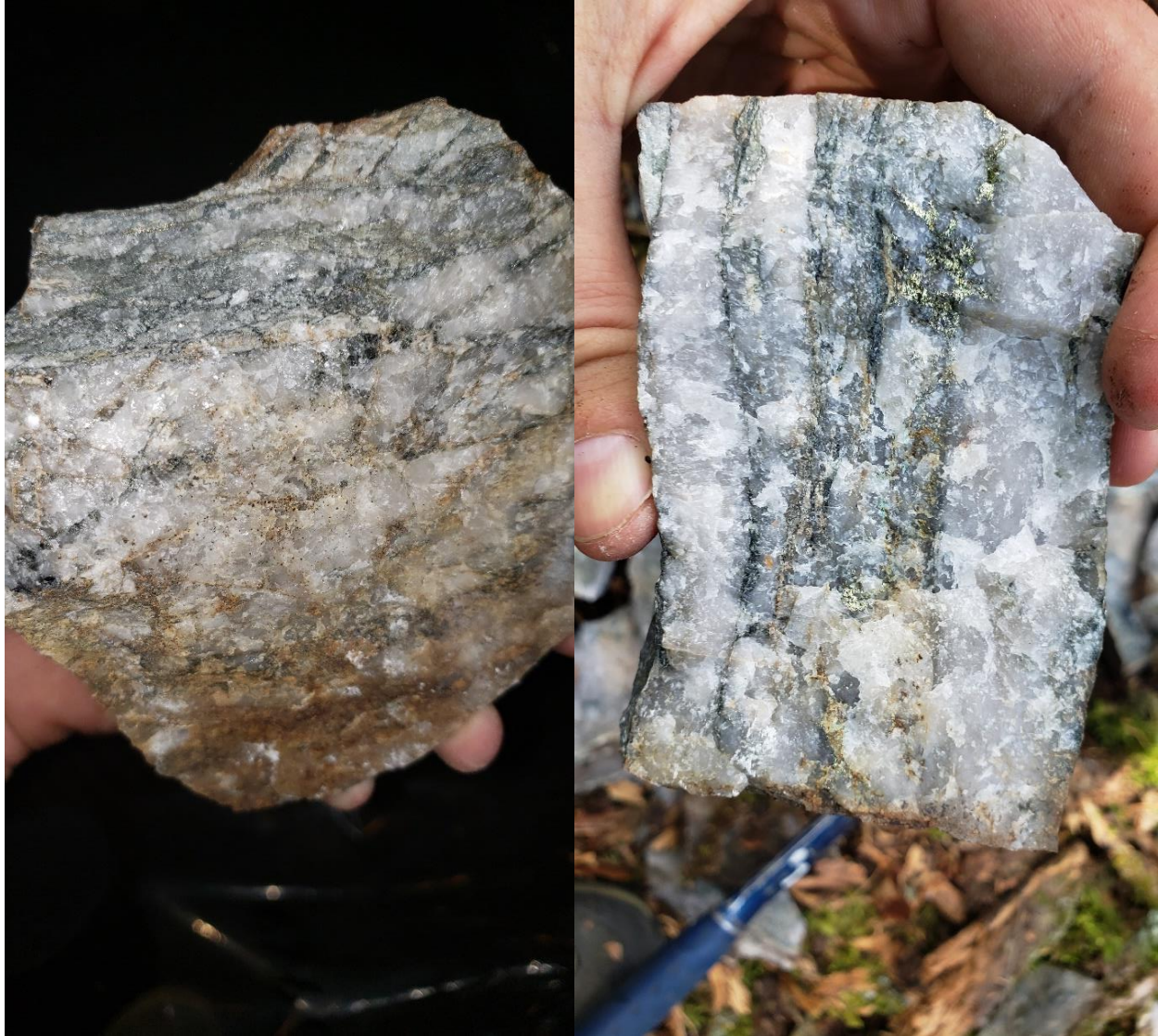
Figure 25: (Left) Sample 75968 with wallrock schlieren/clasts and approximately 5% chalcopyrite; (Right) Sample 75969 with wallrock schlieren and trace amounts of pyrite
