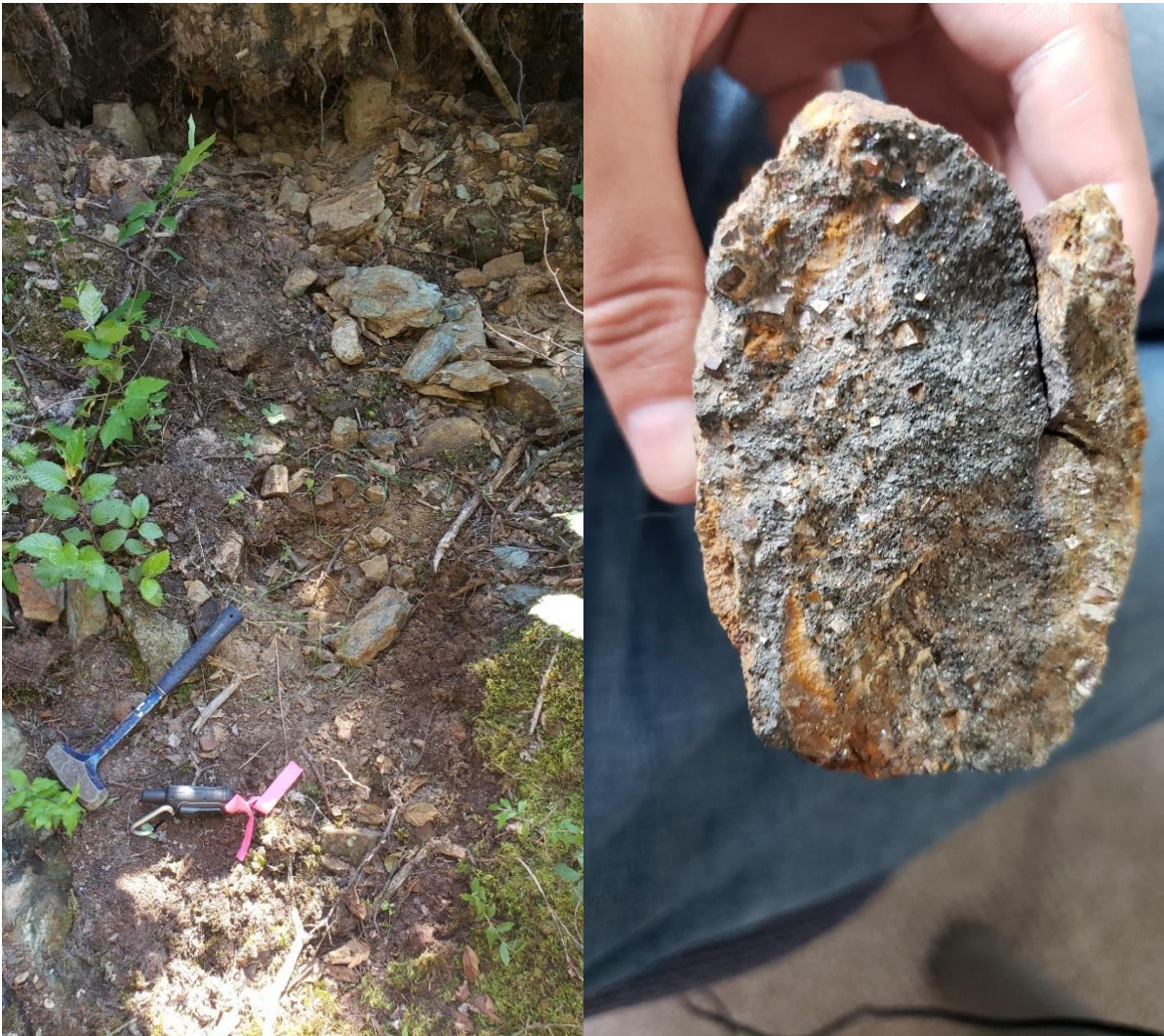
Figure 14. Windfall exposing magnetite-pyrite-rich iron formation. Right: Sample 75951, composed of euhedral magnetite and pyrite in distinct layers
