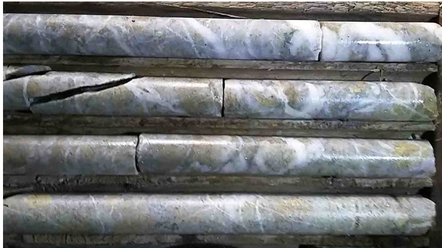
Heavily altered and silicified core from about 20.5 meter depth (core is 22 millimeters in width)
