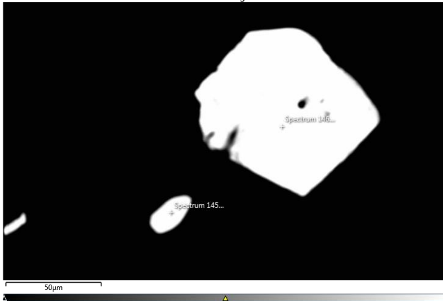
Backscatter image of a grain of Ni-S (vaesite – spectrum 145) and a coarser grain of Ni-As-Sb-Co-S (spectrum 146).
