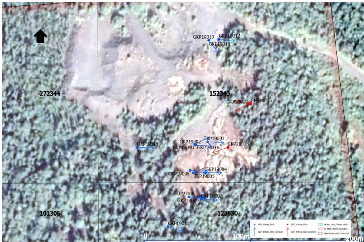
Figure 5. Drill Hole Location Plan- the 3 new 2020 holes are in red and 2018 holes in blue.
