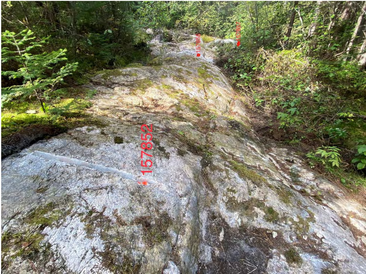
Figure 15-8 Tot Lake pegmatite looking towards north pond with channel samples labelled. TL-CH-20-05 – sample number 157852 TL-CH-20-06 – sample number 157856 TL-CH-20-07 – sample number 157857
