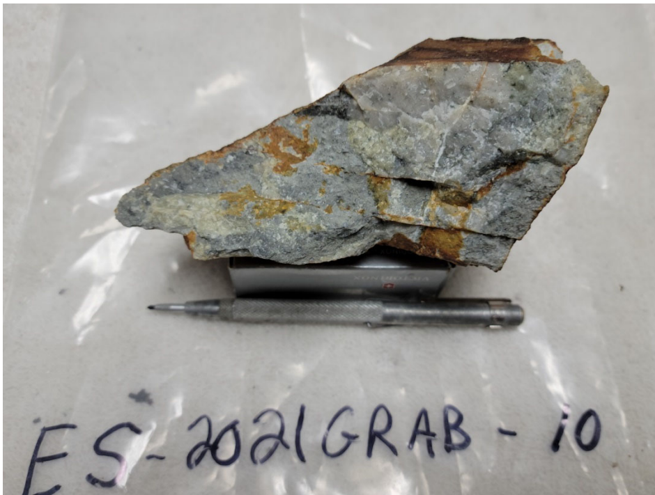
ES-2021GRAB-10: metamorphic/silicified potentially rhyolite with veins/pockets of fine sediment & sulphides (light grey). ES-2021GRAB-10: 0.132gpt Au, 0.4gpt Ag.
