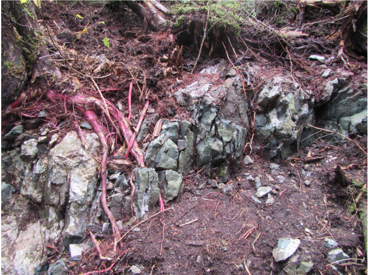
Goldhurst #2 showing (south portion) – quartz carb veinlets with disseminated chalcopyrite/bornite within a medium grey mafic host.
