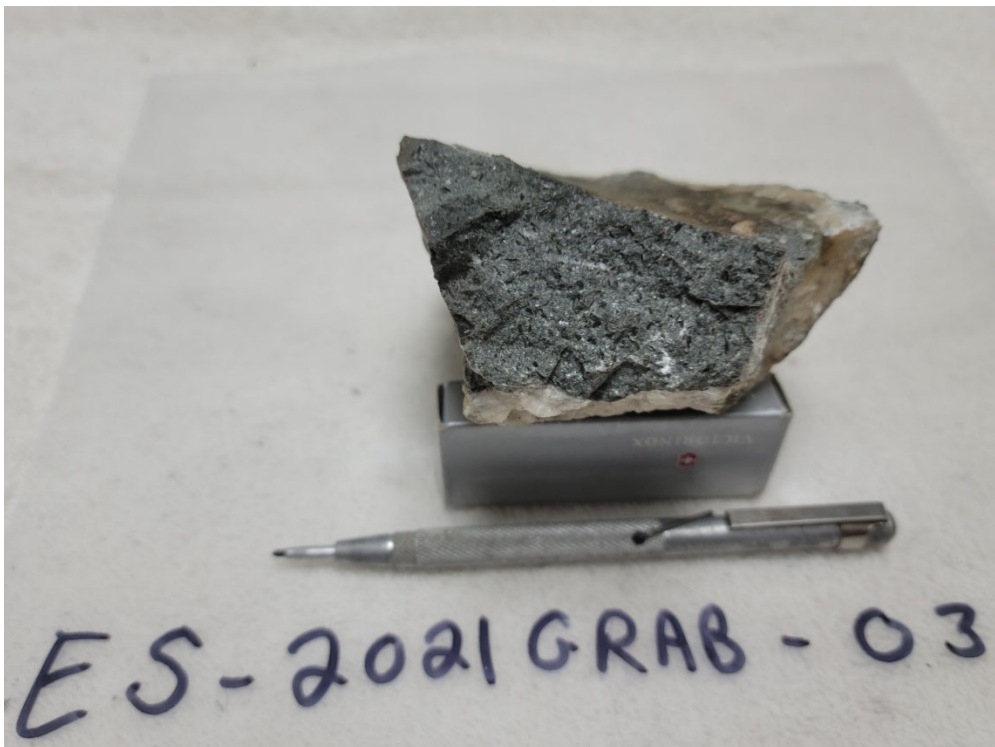
Goldhurst #2 showing – host rock – med grey mafic ES-2021GRAB-03: not sent for assaying
