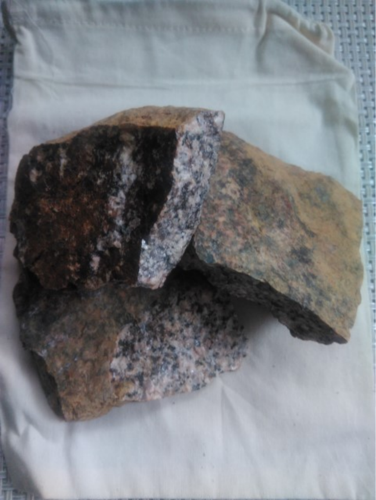
Granite float. Fine-grained; not magnetic. 35% Biotite; 20% quartz; 30% plagioclase; 15% Kspar. Not magnetic, barren of sulfides.
