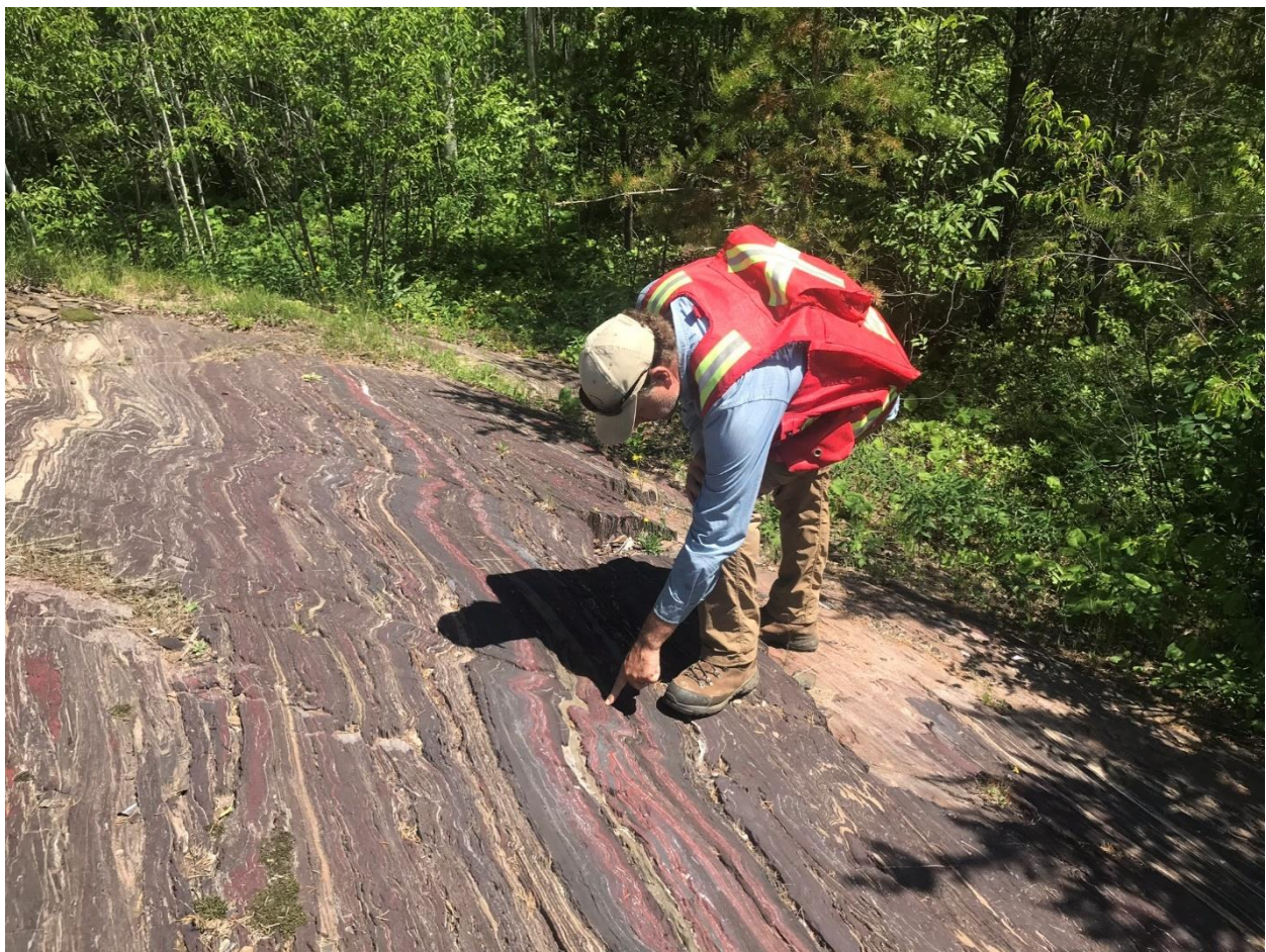
Figure 7: Banded Iron formation found near the Leitch Gold Mine, 1 km NNE of Longrose. This unit extends onto the Longrose project and can easily be delineated on the airborne magnetics survey
