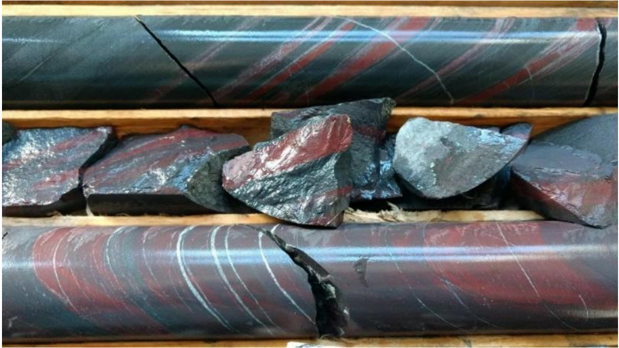
Figure 3: Mingold's 1988 drill core: UND-5 at 335m depth. Logs record black to grey to red, fine grained, hard and well banded 80% magnetite beds and 20% hematitic chert beds. Bedding generally on a 1 to 5 cm scale fine grained specularite associated with hematitic beds (gold 5ppb) with very minor interbedding of clastic sediments. The drill core from this campaign is stored at the Ministry of Mines core library in Thunder Bay.
