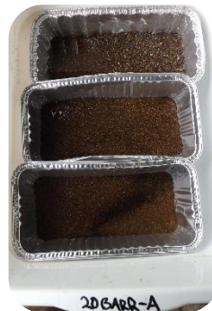
11 – 3 fractions of sluiced cons (0.25-0.5mm, 0.5-1.0mm, 1.0-2.0mm)
