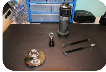
22 – Various rare-earth (N-52) magnets, largest of which is 3" diameter (600lb lift)
