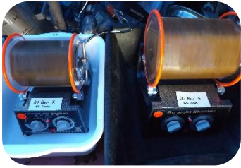
17 – Acrylic tumblers with muriatic acid & different size fractions from the GoldCube. These are variable speed & timers
