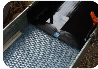
7 – The rubber has a rough surface to slow down and sort grains by size & weight
