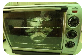
16 – Drying the panned cons – 3 size fractions for each sample
