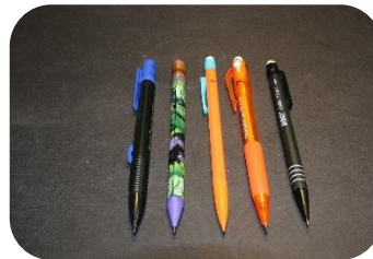
23 – Pencils of varying lead thickness for measuring grains under the microscope
