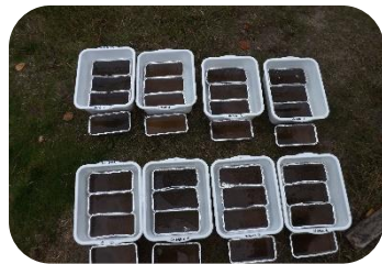
10 – Sluice concentrate screened to 4 sizes before GoldCube
