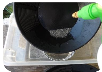
15 – Wash panned cons in aluminum pan for drying
