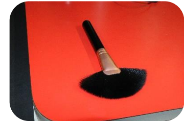
28 – Carbon fibre brush to dissipate electrostatic charge
