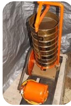
19. Tyler motorized portable sieve shaker
