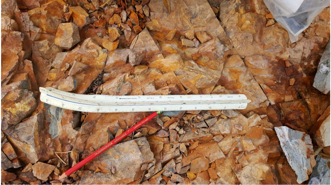
Fig. 8 – Rubbly, oxidized, altered bedrock within the stripping area
