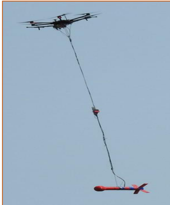
Figure 14. Devbriio UAV-MGtirotor with CS-VL magnetometer.
