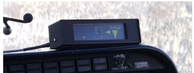
Figure 3. Pilot Steering Indicator and Radio Altimeter Indicator
