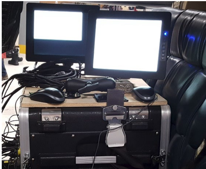
Figure 4. EGL Navigation Computer, Moving-map Display
