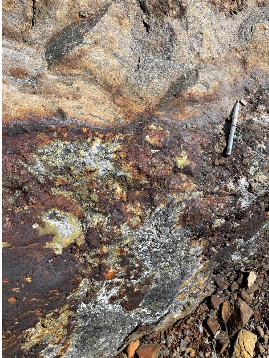
Figure 12 – Photo of quartz vein hosting patchy to semi-massive cpy mineralization located at the contact of the sheared mineral zone and the weakly sheared silicified sandstones to the north. (Rep 5 location)
