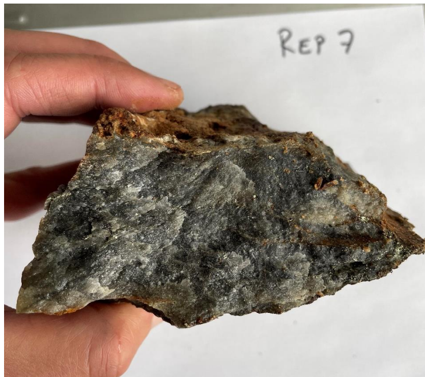
Figure 14 – Photo of Rep 7. Moderately sheared silicified sandstone or potentially conglomerate hosting 3-5% cpy as disseminations and irregular veinlets.
