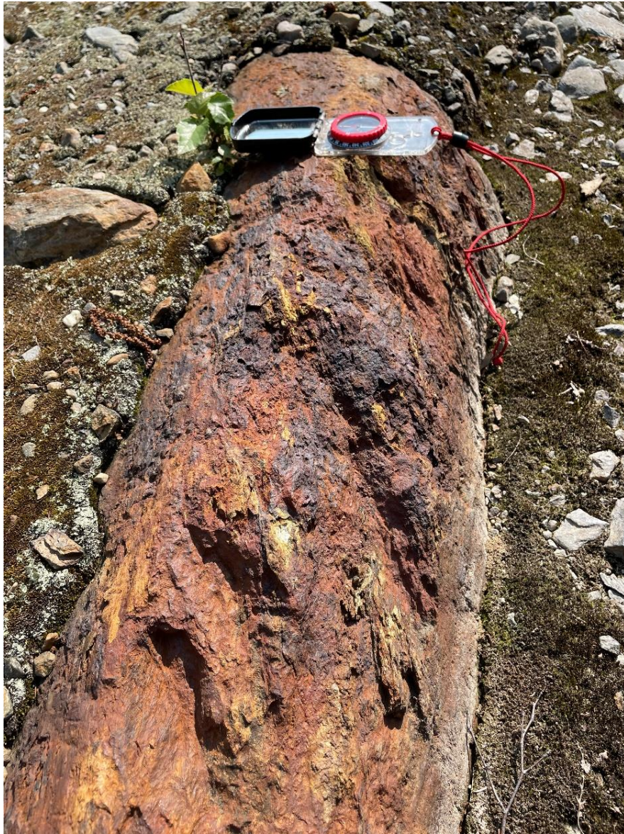
Figure 11 – Photo of the sheared conglomerate within the center of the mineralized zone. Unit is intensely sheared and host to 2-5% cpy as shear-controlled veinlets. (Rep 4 location)
