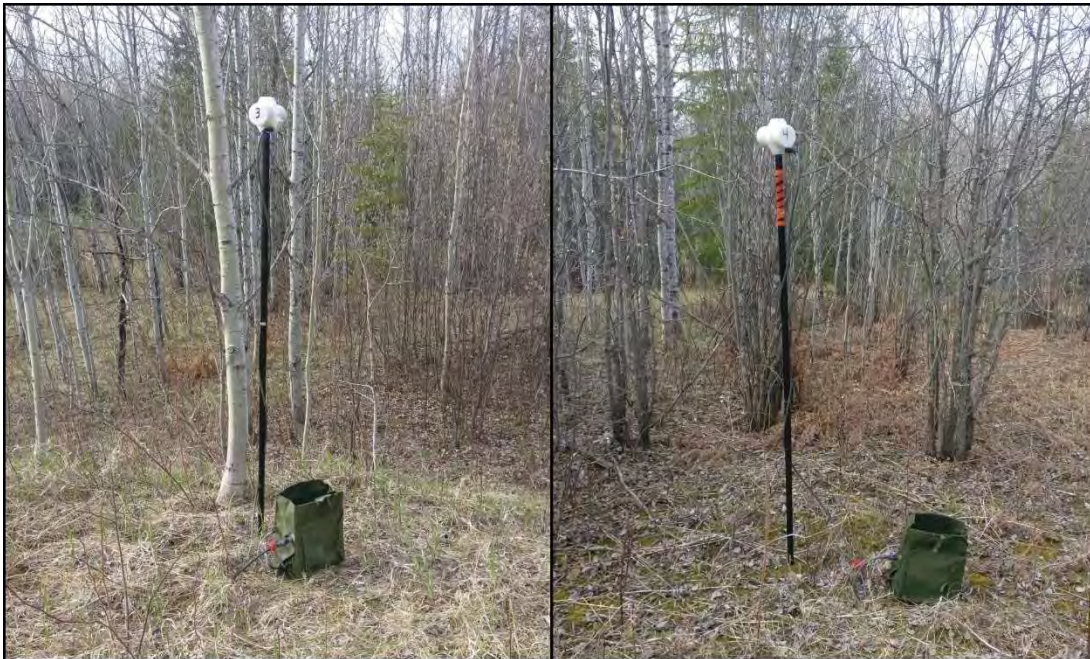
Figure 15: GEM 3 (left) and GEM 4 (right) magnetic base stations west of Matheson, Ontario.
