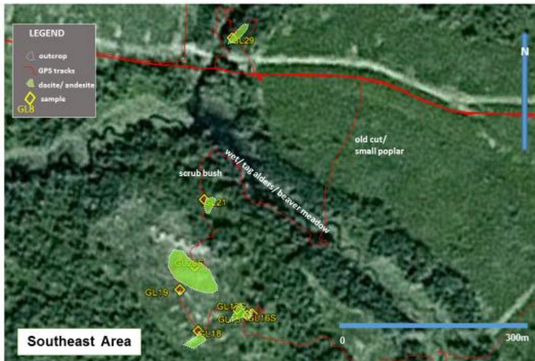
Figure 6: Mapping traverse in southeast area. Note: the photo base from Google Earth does not match the GPS tracking coordinates exactly, but falls approximately 30m to the south
