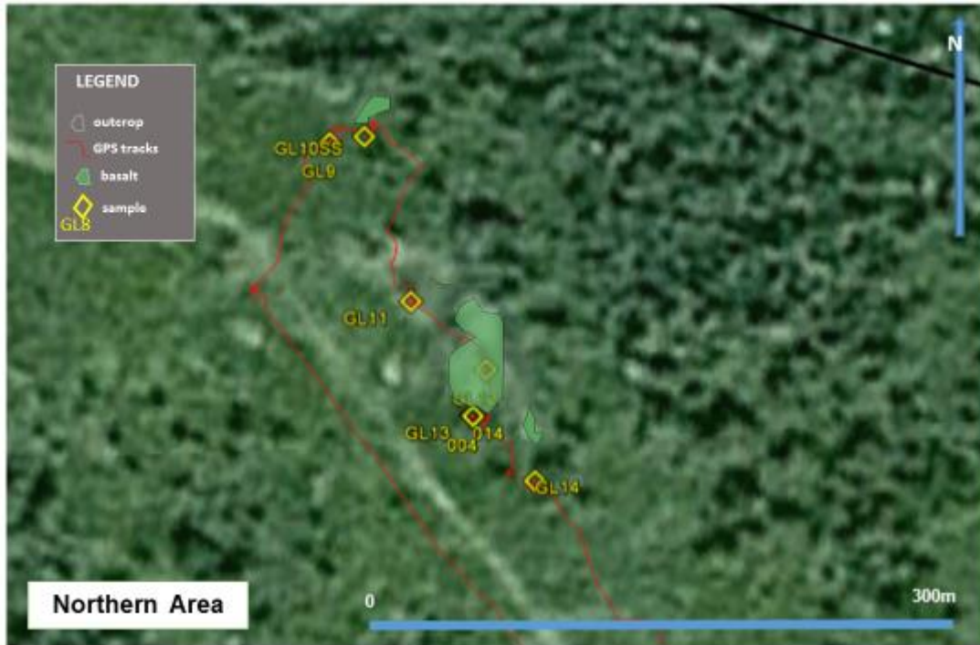
Figure 5: Mapping traverse in Northern area. Note: the photo base from Google Earth does not match the GPS tracking coordinates exactly, but falls approximately 30m to the south
