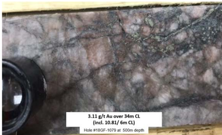
Photograph 2: sawn surface of NQ core showing the breccia pattern of deformation observed in hole #18GF-1079 and the later-stage pyrite enhancement of the fractures
