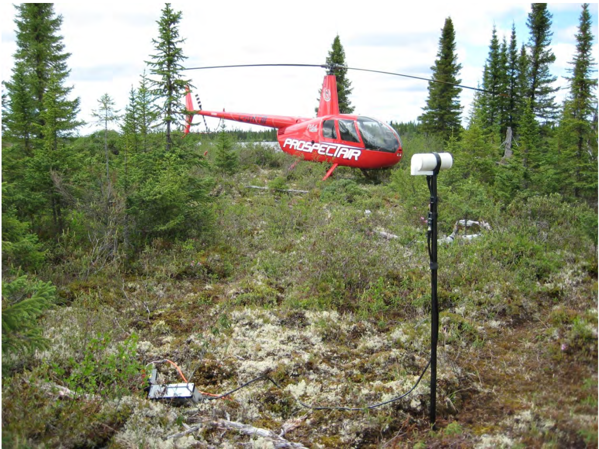
Figure 5: Example of a magnetic base station setup
