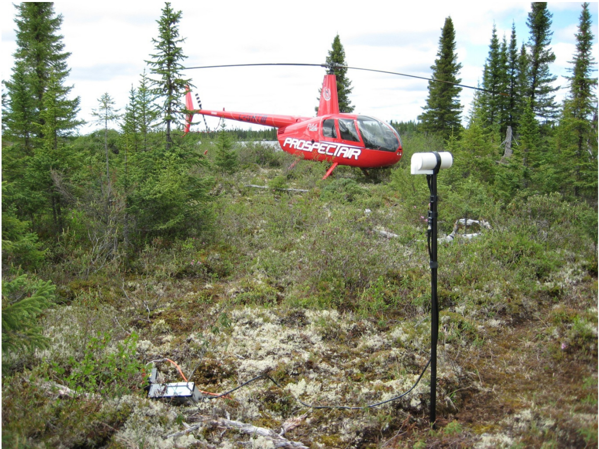
Figure 5: Example of a magnetic base station setup
