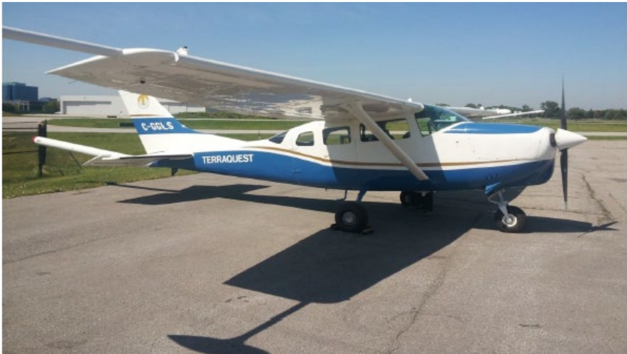
Figure 9: Survey Aircraft- Cessna U206 with sensor arrays
