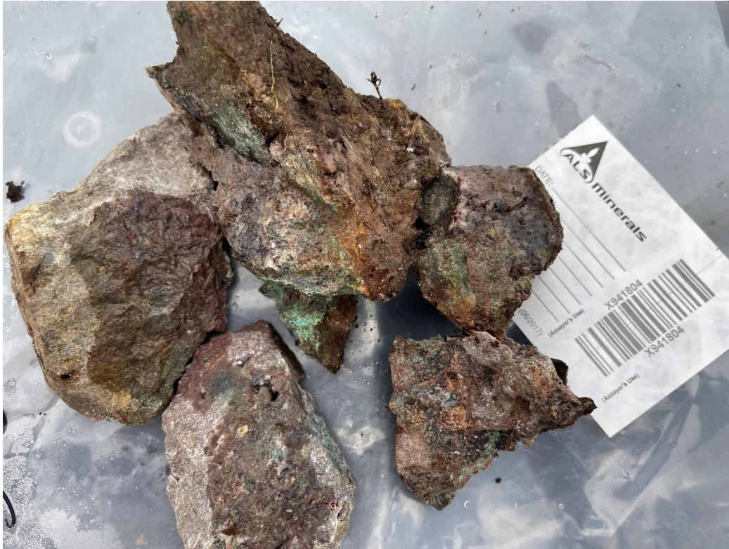
Figure 11: X941804 – rubble beside shaft – 2.14 g/t Au, 36.9 g/t Ag, 1.33% Cu, 1050 ppm Ba, 436 ppm Zn, 222 ppm Bi
