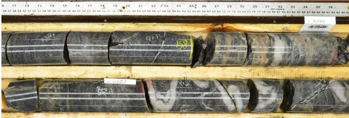
Figure 7-11: Brittle-ductile shearing and tight folding of auriferous quartz veins in the Jubilee Shear Zone
