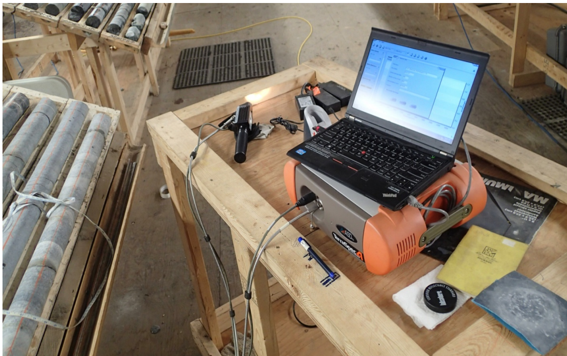
Figure 10-3: TerraSpec 4 Hi-Res Mineral Spectrometer and data acquisition computer on the rolling table used to acquire SWIR data on historic core
