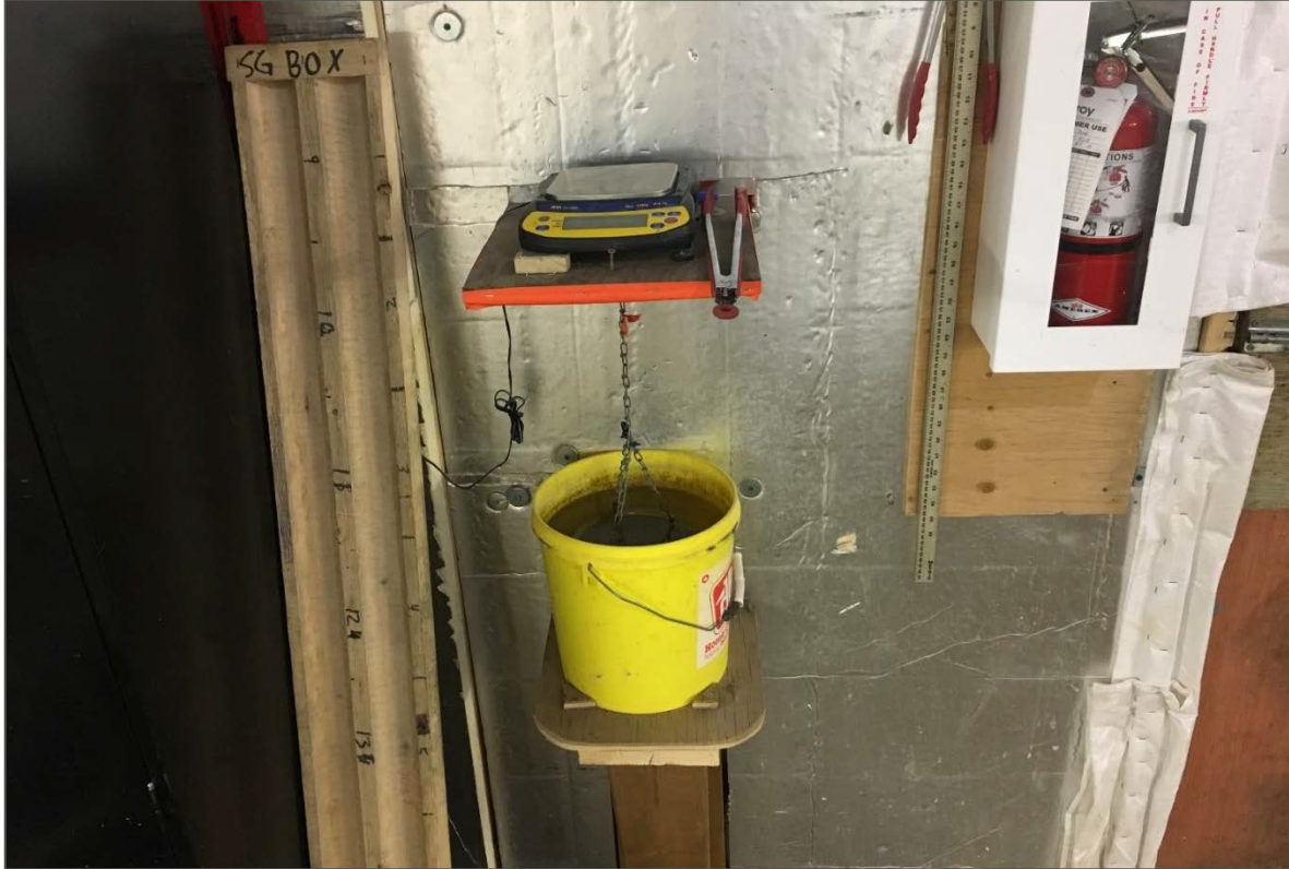
Figure 10-4: SG Measurement at Red Pine's Core Logging Facility
