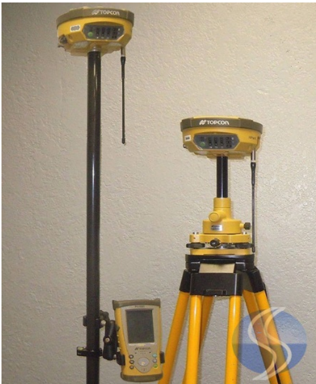
Figure 9-11: TopCon RTK GPS used to get precise location of the channel samples
