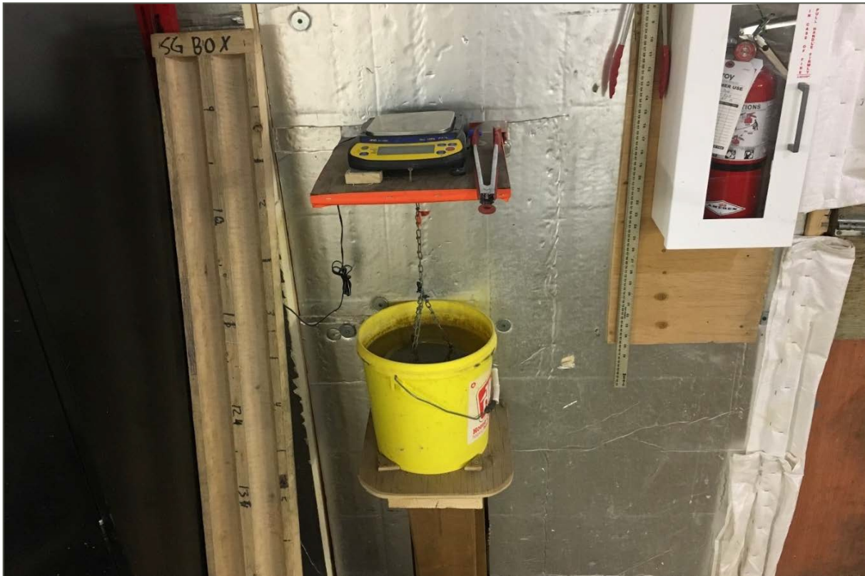
Figure 11-2: SG measurement at Red Pine's core logging facility
