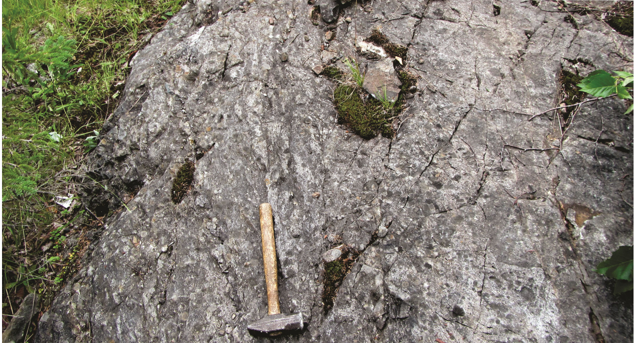
Figure 7-17: Shear zone hosting the Cooper Vein characterized by brittle-ductile shearing preferentially partitioned at the contact between the medium- to coarse-grained diorite and porphyritic units
