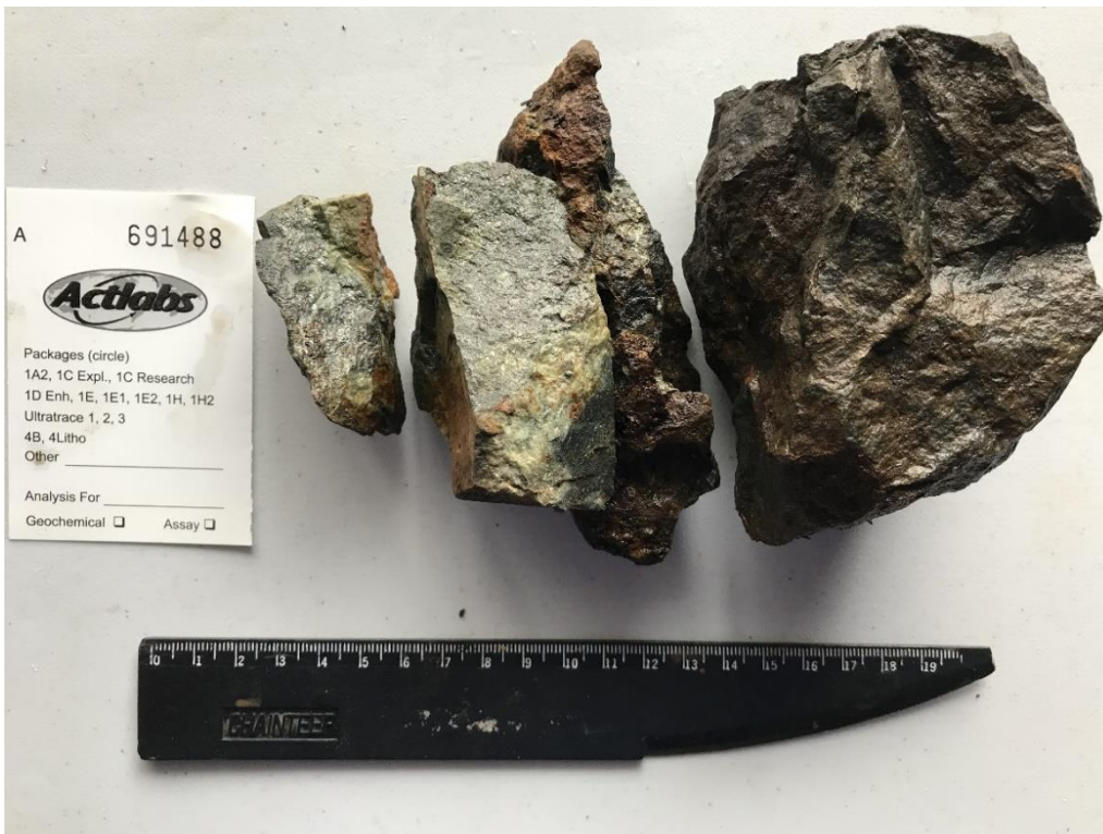
Figure 12: 691488 – 0.139 g/t Au, 1.37 g/t Ag, 489 ppm Co, 755 ppm Cu, 278 ppm Ni, 15.35 ppm W, 4.93 ppm Te
