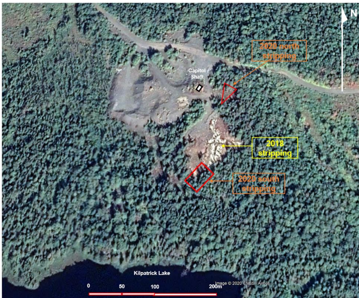
Figure 4. Location of 2020 stripping with respect to original 2018 stripped area of the Kilpatrick cobalt vein (former Capitol minesite, Gowganda area).
