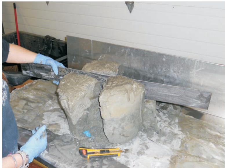
b) The block is quartered and thin slices are removed from a random quarter until the desired split size is achieved.
