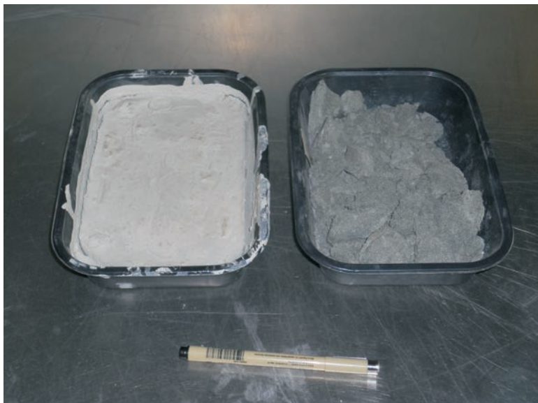
c) Typical appearance of silt-rich (left) and sandy (right) tailings sample splits after drying.
