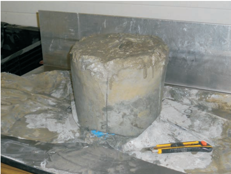
a) Example of a sample of water-saturated, silt-rich tailings compacted into the cylindrical form of the shipping pail.
