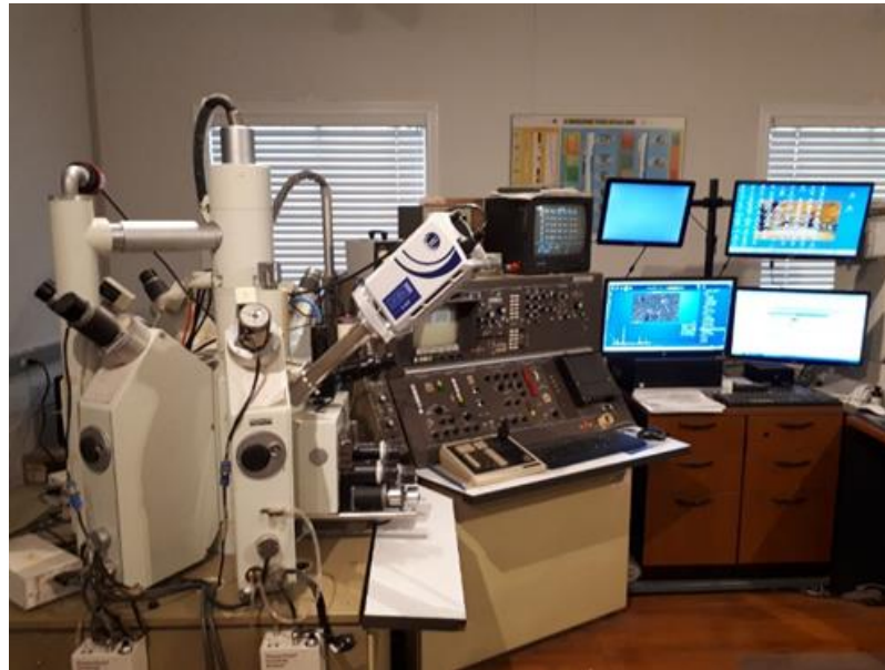
Figure 7 JEOL JXA-733 Superprobe equipped with an Oxford Xact EDS system housed in the Laboratory of Renaud Geological Consulting Ltd.
