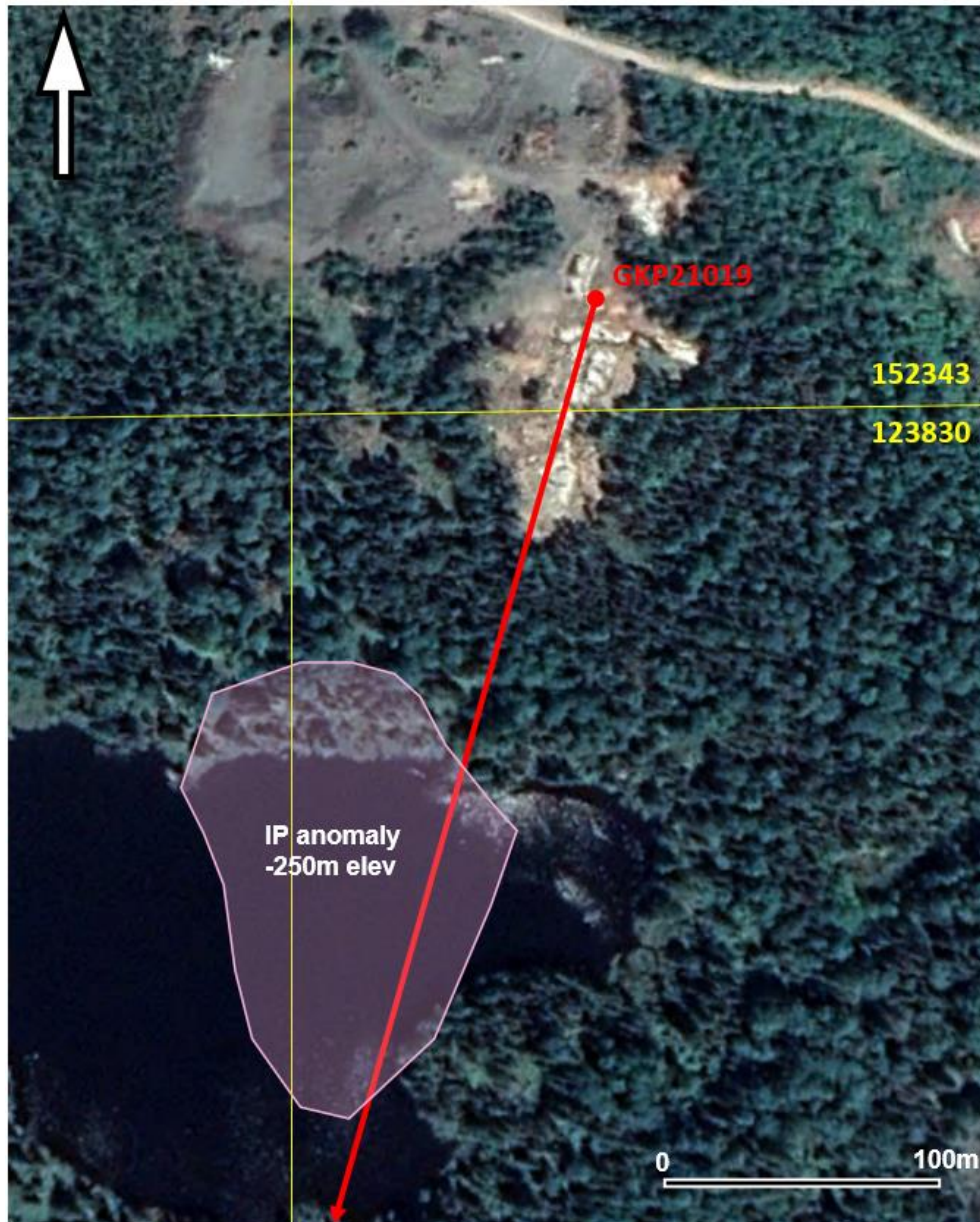
Figure 5. Drill Hole Location Plan- hole GKP21019 in red, IP chargeability anomaly at -250 elevation in pink.
